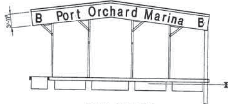
END VIEWS B FLOAT [52-FOOT COVER SHOWN] [28-FOOT COVER SIMILAR]
